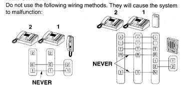
Do not parallel sub station wires between TB-M master stations. Wiring from TB-SE must be homerun to EACH master station.
